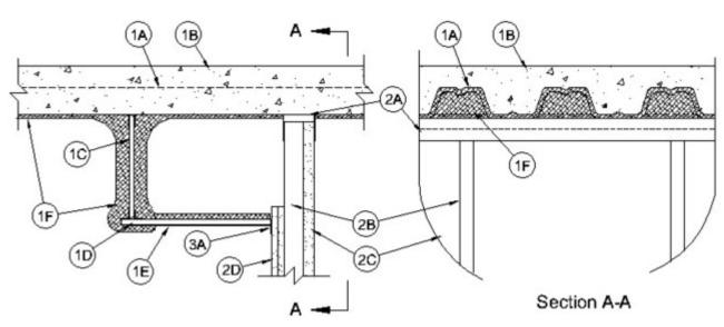
1. **Floor Assembly** — The fire-rated fluted steel deck/concrete floor assembly shall be constructed of the materials and in the manner described in the individual D700 Series Floor-Ceiling Design in the UL Fire Resistance Directory and shall include the following construction features:
