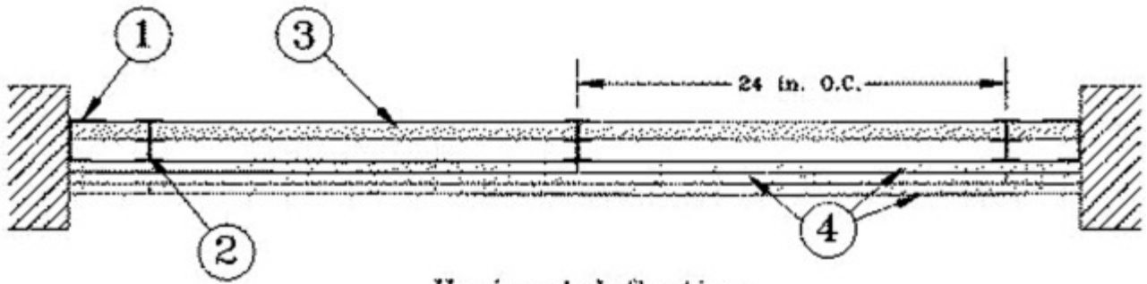
Horizontal Section System H - 3 Hr.
