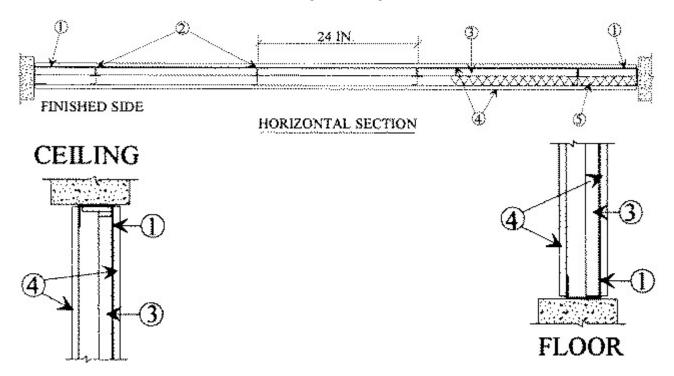
1. **Channel Track** — "J" shaped channel, 2-1/2 in. wide with unequal legs of 1 in. and 2 in., fabricated from 25 MSG galv steel channel attached to structural supports with steel fasteners located not greater than 2 in. from ends and not greater than 24 in. OC.
