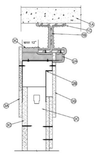
1. **Floor Assembly** — The 1 or 2 hr fire-rated concrete floor assembly shall be constructed of the materials and in the manner described in the individual J700, J800 or J900 Series Floor-Ceiling Design in the UL Fire Resistance Directory and shall include the following construction features:
