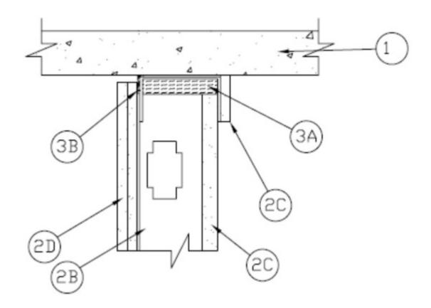
1. Floor Assembly - Concrete - Min 2-1/2 in. (64 mm) thick reinforced concrete.
