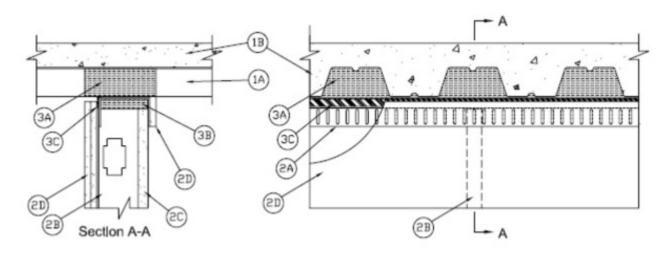
1. **Floor Assembly** — The fire-rated fluted steel deck/concrete floor assembly shall be constructed of the materials and in the manner described in the individual D900 Series Floor-Ceiling Design in the UL Fire Resistance Directory and shall include the following construction features:
