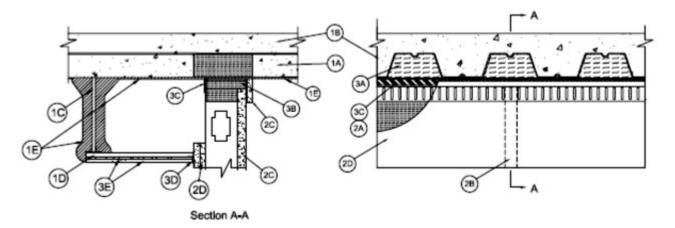
1. **Floor Assembly** — The fire-rated fluted steel deck/concrete floor assembly shall be constructed of the materials and in the manner described in the individual D700 Series Floor-Ceiling Design in the UL Fire Resistance Directory and shall include the following construction features:
